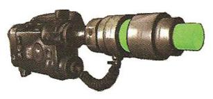
"Laser light" pointer tool: This handheld device was designed as a simple "point and shoot" tool that assists in locating and tracking a variety of nonorganic chemical substances by altering the frequency and intensity of the laser beam, causing specified chemicals or
